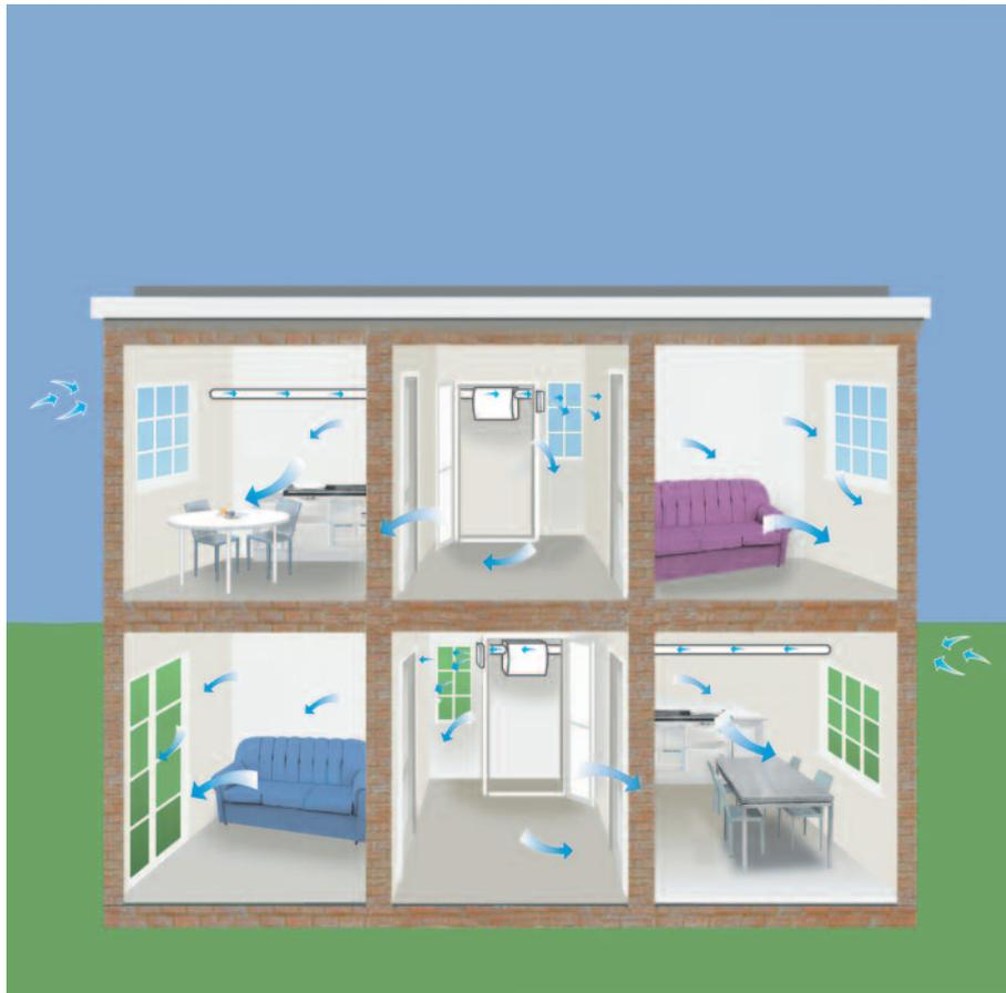
■ The Flatmaster is fitted on a wall within your property to ventilate your home. Fresh air will be drawn from outside, filtered through the fan unit and then supplied into the central hallway through a grille.
