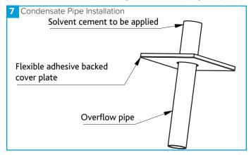
The condensate must be discharged under a water level in a U-trap drainpipe or an alternative drain method which acts as an airlock. This condensate discharge connection is suitable for 21.5mm Ø overflow pipe. Solvent cement should be used to make the joint.
