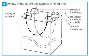
If the MVHR unit has integral automatic HX bypass (AB models only), the bypass damper shall open automatically via a wax actuator allowing the air to bypass the heat exchanger to deliver fresh filtered air during the warmer months.
