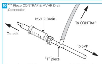
When using a "T" Piece to connect the CONTRAP drainage and the MVHR drain pipework the MVHR drain must always be fitted before the "T" Piece to prevent condensate from feeding back into the MVHR system.
