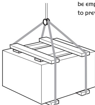
Figure 1. Lifting unit with slings via spreaders.
