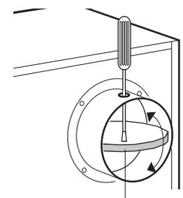
When spigot is in position, damper can be adjusted using a screwdriver.
