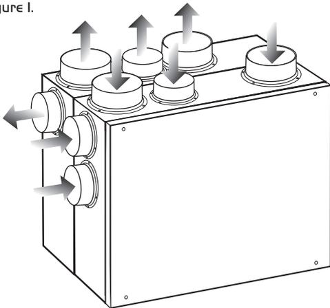
The unit is fitted with two independent fans. Each fan has full speed control for background and boost ventilation rates as well as a run-on timer facility. To recover heat from the extract air an aluminium heat exchanger block is utilised. This heat exchanger can recover over 70% of the normally wasted heat.
