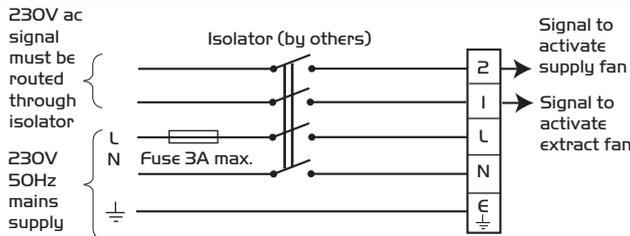
The unit is designed to be wired directly to the mains supply through a fused spur isolator (by others). With the rear section only fixed in position bring the mains wiring through the cable gland in the base of the unit (this gland can be moved to the side position if required).
