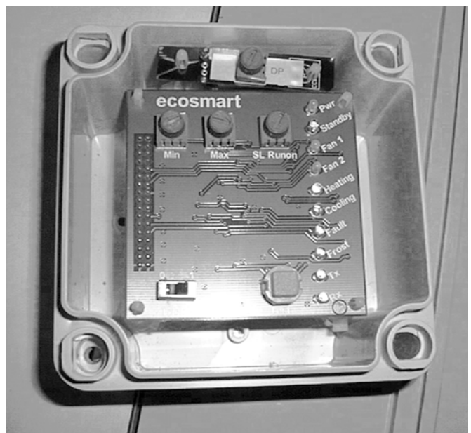
Figure 5. Fan side commissioning box.
