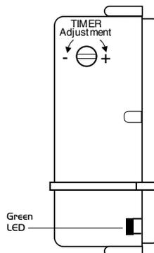
The Genie-MS will activate only when 230V is presented to the brown wire and 230V is presented to the black wire (Via light switch, door switch).
