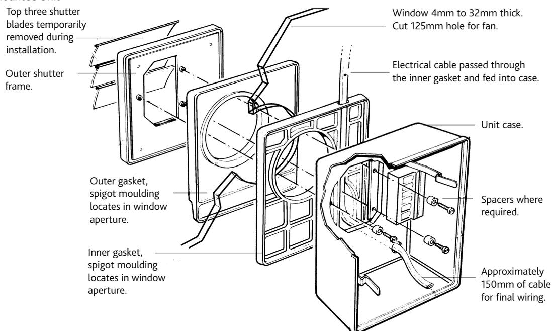
The window mounting kit (WINKIT) is designed for mounting the unit into windows 4 mm to 32 mm thick using a 125 mm Ø hole (Figure 9).
