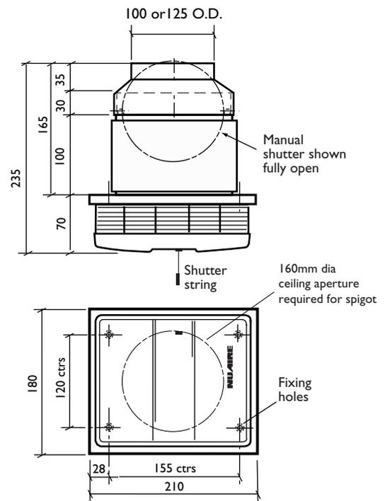
Fig. 3. Dimensions and fixing details
