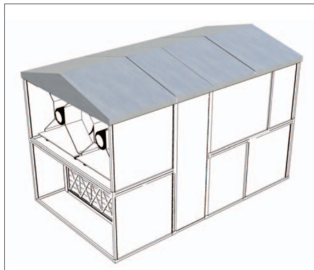
Figure 12 Installed weatherproof roof components.
